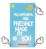
Evacuate all water from the reservoir and evaporator by entering the Service screen> Service Outputs> Cleaning and toggling the Ice Maker Dump Valve ON until all water has been emptied from the system then toggle OFF.
