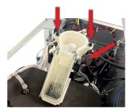
14. Using a clean pitcher/cup pour the sanitizer solution into the top of the evaporator unit full, any excess will exit through the overflow tube in the reservoir.
