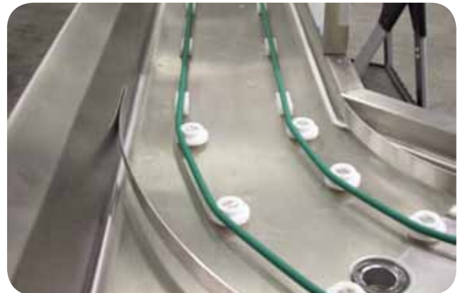
Poly Cord with UHMW guide blocks and wheels
